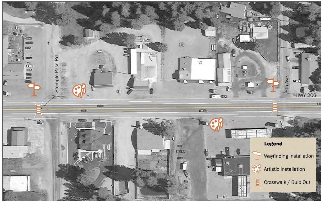
Figure 34. Crosswalks, bulb outs, wayfinding, artistic installations, and should striping are depicted in the graphic above at Main Street's intersection with Stemple Pass Road and 6 th Avenue.
