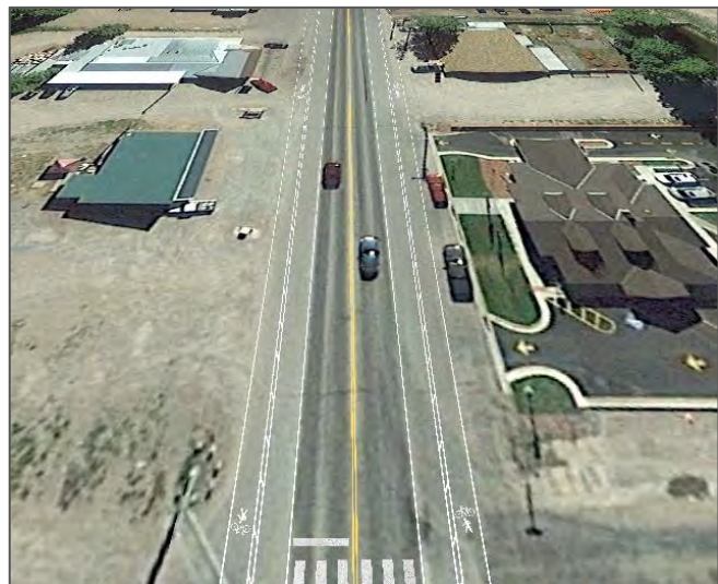
Figure 31. Paved shoulder design created by the Master Plan Steering Committee and MSU CDC.
